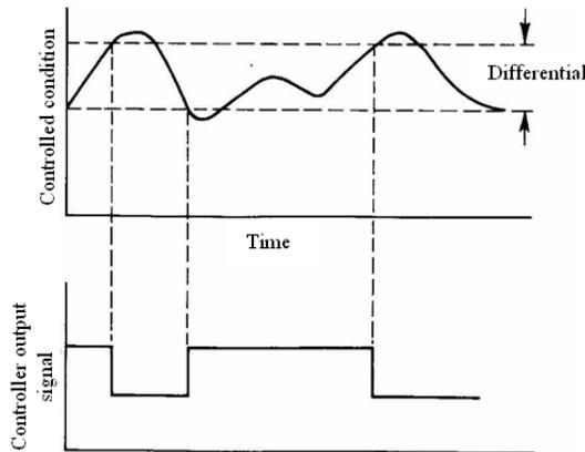
Fig. 3: Action of an on/off controller
