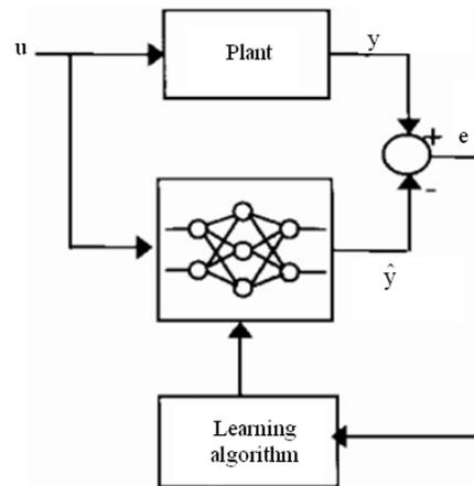
Fig. 6: Forward system identification
