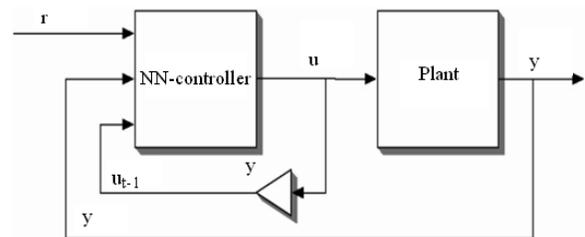
Fig. 8: Direct neural network controller
