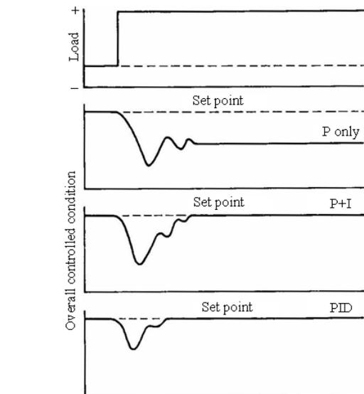
Fig. 4: Action of a PID controller
