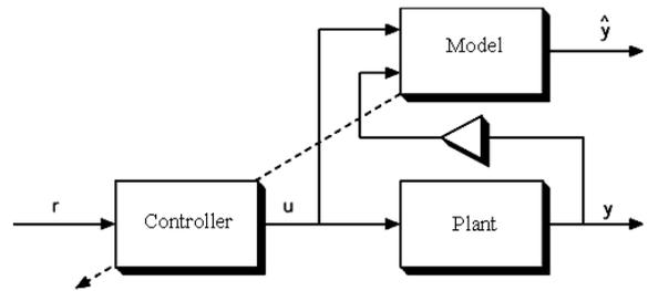
Fig. 5: Neural Network based Predictive Controller
