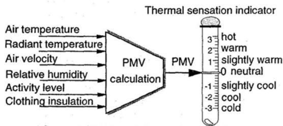
Fig. 1: PMV index and thermal sensation indicator (Fanger model)
