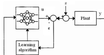
Fig. 7: Direct inverse system identification
