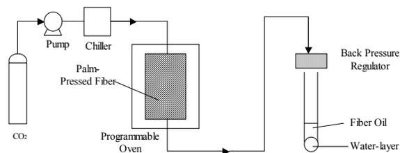
Fig. 1: Schematic diagram of SC-CO<sub>2</sub> extraction system
