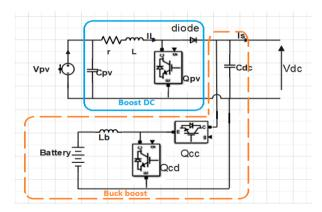
Fig. 3: DC-micro grid system circuit for stability analysis
