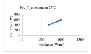
Fig. 13: Variation of PV power with irradiance when Temperature is constant
