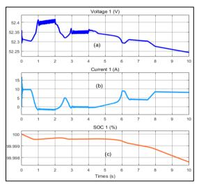
Fig. 18: State of the battery household 1; a: Voltage; b: current; c: State of charge
