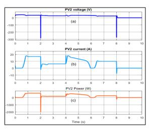
Fig. 16: Characteristics of PV2; a: PV2 Voltage (V); b: PV2 Current (A); c: PV2 power (W)
