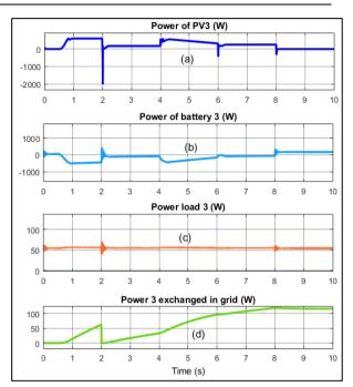
Fig. 24: Characteristics Power of household 3; a: PV power; b: Battery power; c: Load power (W); d: Power 3 exchanged
