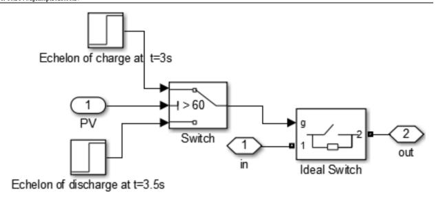
Fig. 6: The interconnect source control process
