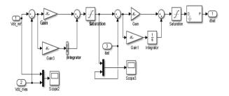
Fig. 4: PI command simulated in Simulink
