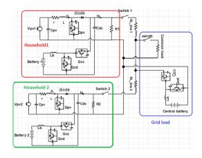
Fig. 2: Electrical model of micro-grid
