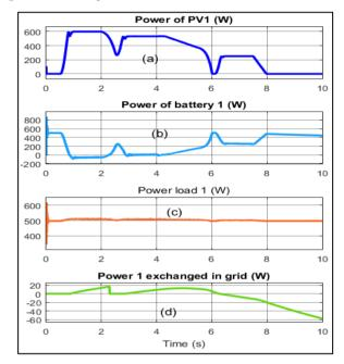
Fig. 22: Characteristics Power of household 1; a: PV power; b: Battery power; c: Load power (W); d: Power 1 exchanged
