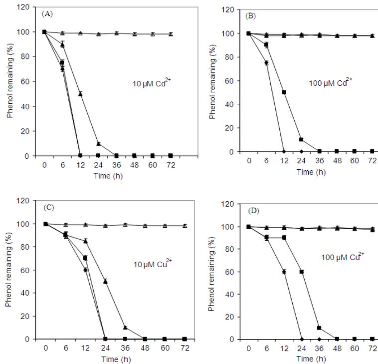
Fig. 2: Effect of cadmium and copper concentrations on the phenol utilization by *Pseudomonas putida* PhCN and its derivatives. Strains symbols: (◆): PhCN without Metals (control); (■): PhCN; (▲): PhCN1; (△): PhCNM
