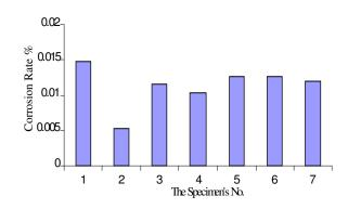
Fig. 2: Corrosion rate in the aquarium
