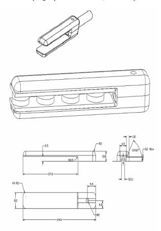
Fig. 6: Endoscope grasper mounting with the sensors and its detailed drawings. Dimensions are in mm.
