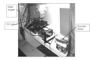
Fig. 5: Photolithography set-up.
