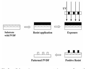
Fig.3: Schematic representation of the photolithography process.
