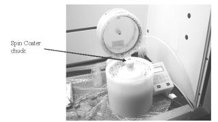
Fig. 4: Photograph of the spin coater set-up.
