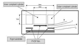
Fig. 1: Schematic representation of the sensor unit.
