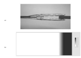
Fig. 8: a) Photograph of the endoscopic grasper touching an elastomeric object (with softness of 43 Shore). b) The softness display shows the object in gray scale.
