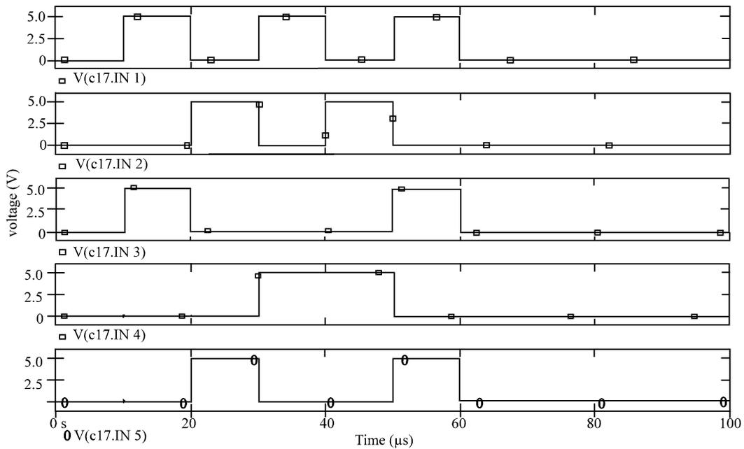
Fig. 3: 60 μs Input Waveform for the Benchmark Circuit "c17"
