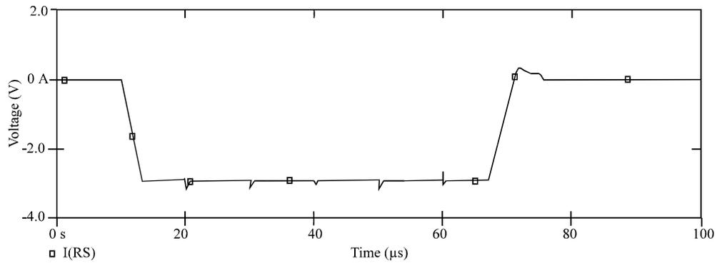
Fig. 6: Simulation Results Showing Fault-free  $I_{\text{DDQ}}$  without VCS
