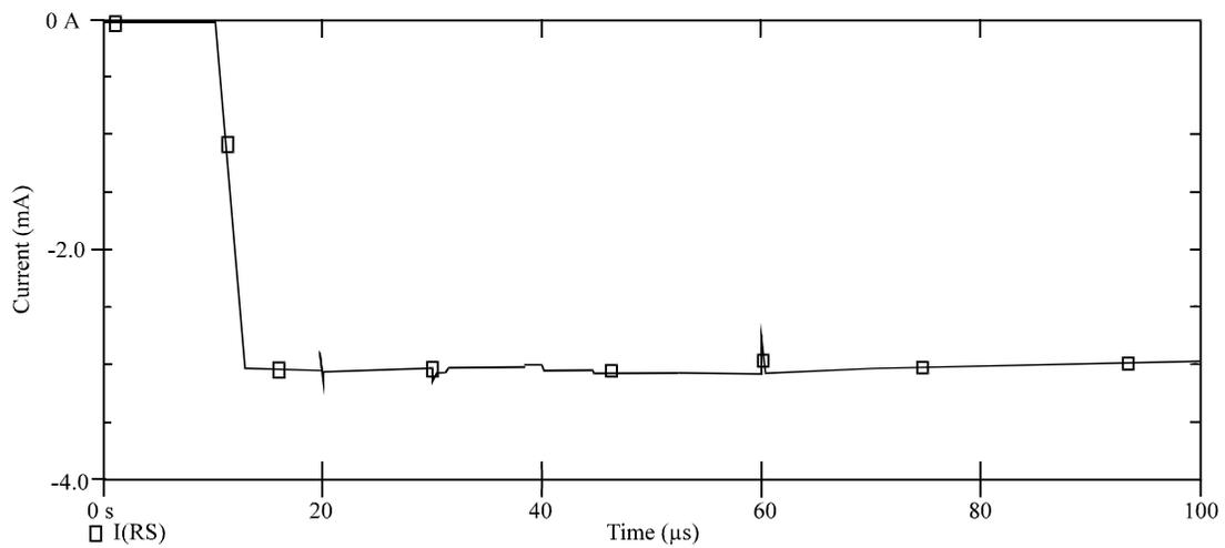
Fig. 7: Simulation Results Showing Faulty  $I_{\text{DDQ}}$  Without VCS
