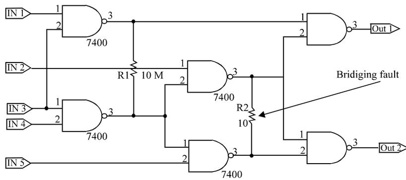
Fig. 2: c17 Benchmark Circuit with Bridging Faults Between Two Logic Elements
