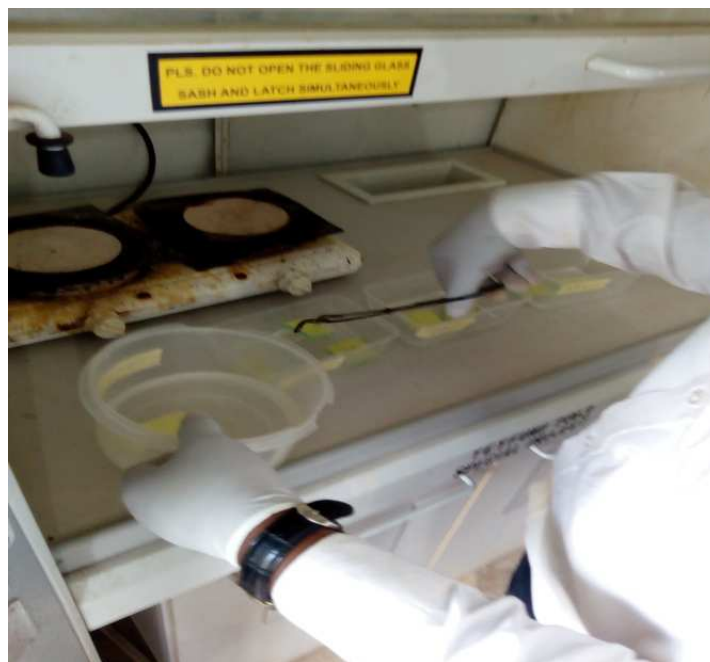
Fig. 2: Acid etching process in fume cupboard
