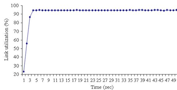
Fig. 5: Link utilization for bottleneck link with four flows
