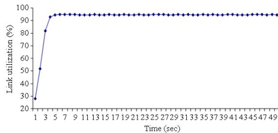
Fig. 4: Link utilization for bottleneck link with three flows
