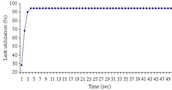
Fig. 6: Link utilization for bottleneck link with five flows
