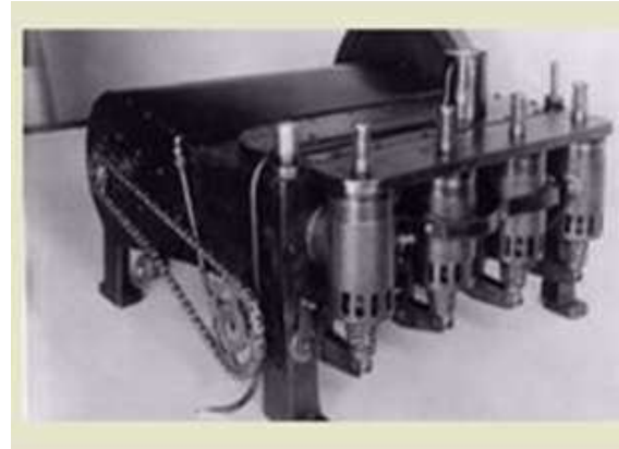
Fig. 2. The engine Wright Source: https://airandspace.si.edu/exhibitions/wrightbrothers/online/fly/1903/engine.cfm
