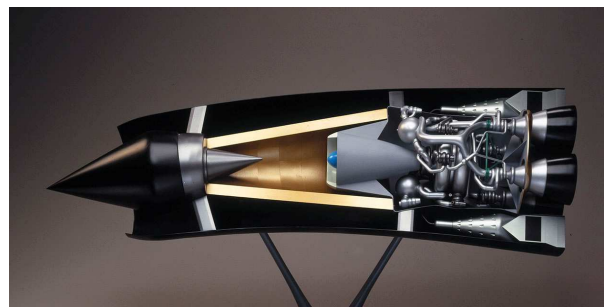
Fig. 7. The Saber (or Sabre) engine is a hybrid between aerobic engine and rocket engine
