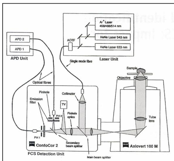
Fig. 1: Fluorescence Correlation Spectroscopy (FCS). The laser beams are focused to small spots in the sample solution. The fluorescence light is collected by the objective and passes through the beam splitter which reflects the excitation light into the objective and transmits the fluorescence light from the sample. Fluctuations in the fluorescence light are detected by photo diodes.
