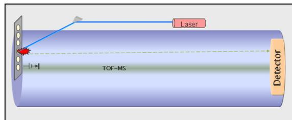
Fig. 2: Surface enhanced laser desorption ionisation time of flight (SELDI-TOF). The proteins are “eluted” from the matrix array by laser desorption. The masses of the ionized proteins are accurately determined by Time-of-Flight Mass Spectrometry.
