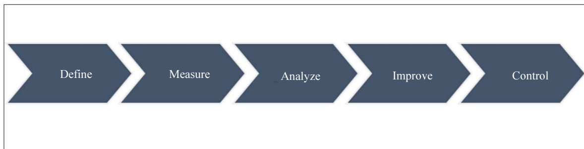
Fig. 1: Phases DMAIC; Define: Develop the scope of the team’s work, define the macro map of the process, select customer requirements and analyze resistances; Measure: Map the process, analyze opportunities for process simplification, plan data collection, validate the measurement system and establish process capacity; Analyze: Analyze the chances of process redesign and identify the root causes that affect its performance; Improve: Advanced analysis of causes, find solutions, pilot and plan implementations of desired solutions; Control: Design new controls, conclude implementations and calculate their ability to analyze whether the result was achieved
