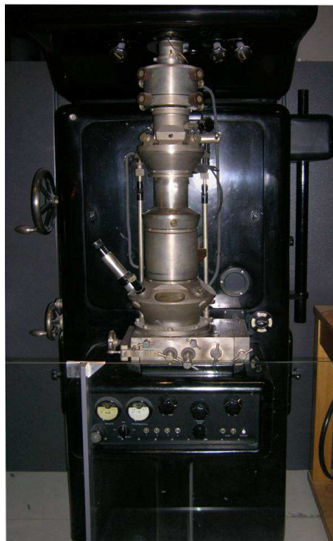
Fig. 2. Electron microscope constructed by Ernst Ruska in 1933; Source: https://en.wikipedia.org/wiki/Ernst_Ruska
