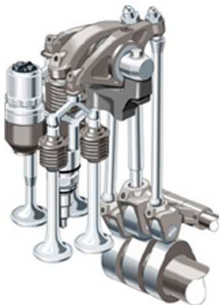
Fig. 10. The Scania distribution mechanism
