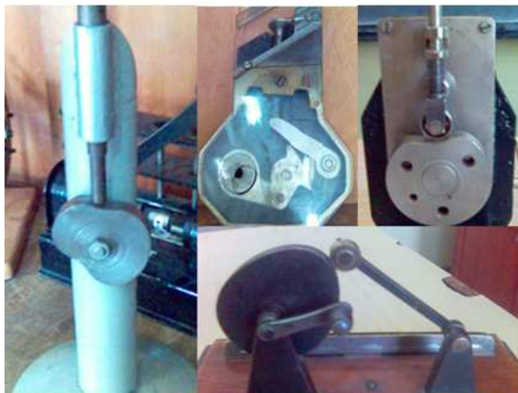
Fig. 3. Mechanisms with rotary cam and follower
