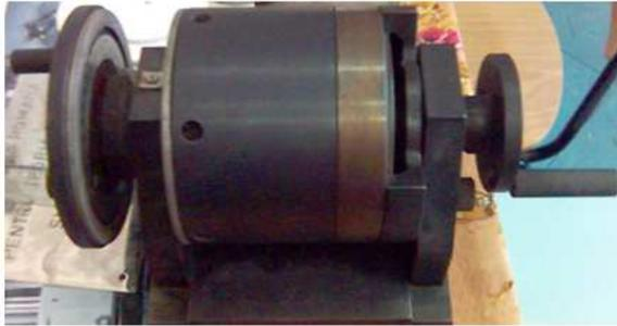
Fig. 1. Constructive photo of a harmonic drive
