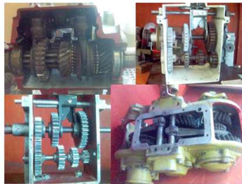
Fig. 10. Some manual gearboxes used in road vehicles
