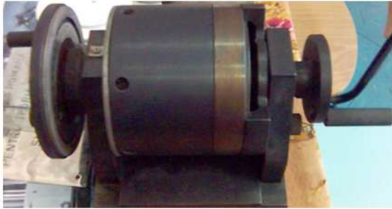
Fig. 1. Constructive photo of a harmonic drive
