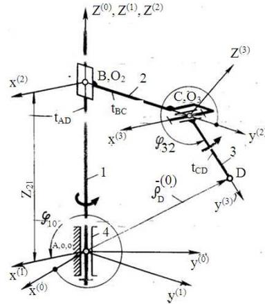
Fig. 3: Schematic representation of the rubbish prickling mechanism<sup>[1]</sup>
