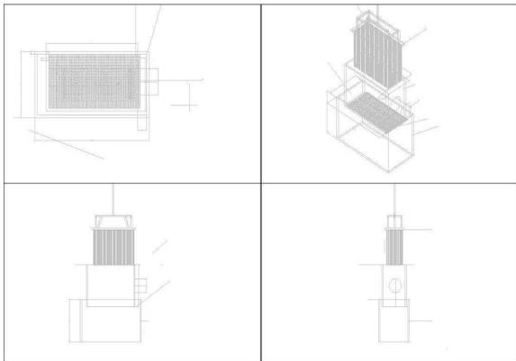
Fig. 2b: Sketch of the Rubbish Pickling Machine (in Three Views and Isometric)
