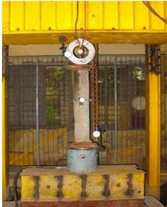
Fig. 3: Column test setup and instrumentation
