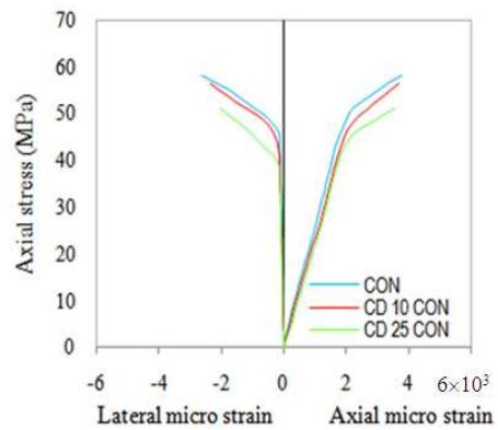
Fig. 5: Stress-strain response of columns
