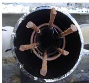
Fig. 1: Reinforcement cage in formwork
