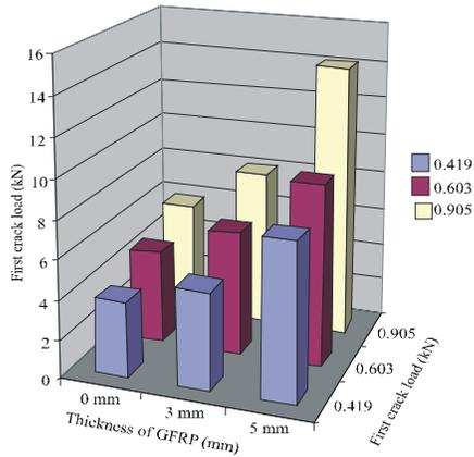
Fig. 2: First crack loads
