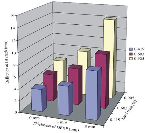
Fig. 5: Deflection at first crack
