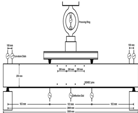
Fig. 1: Loading and Instrumentation Setup
