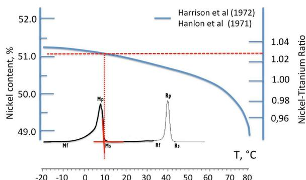
Fig. 4. Detail of DSC characterization of the NiTi alloy composition in the cooling stage
