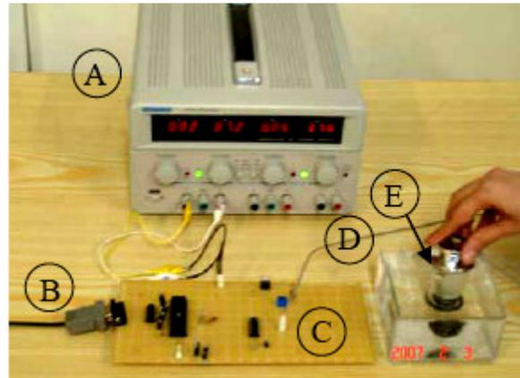
Fig. 10: Experimental setup: A- power supply, B- serial port, C- electronic board, D- simulated tissue and tumor, E- tactile probe.
