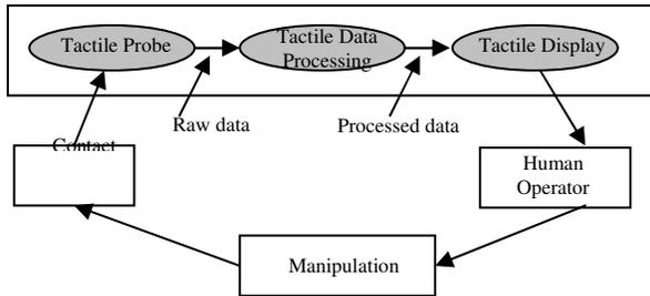
Fig. 9: Components of the *Tactile Tumor Detector*
