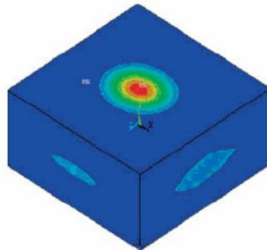
Fig. 4: Elliptical stress contours for an oval tumor (Oval: *l, 5mm; t, 5cm; d, 4cm; h, 2.5cm; Er, 30*).
