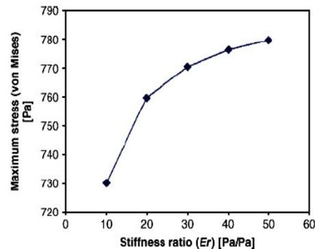
Fig. 8: Tactile Map of maximum stress vs. stiffness ratio
