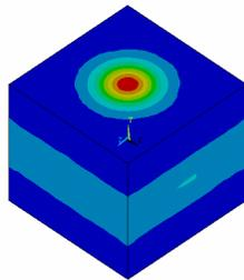
Fig. 2: Tactile Image for the code (Sphere: *l, 5mm; t, 8cm; d, 2cm; h, 4cm; Er, 30*).
