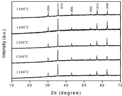
Fig. 1: XRD patterns of MZF ceramics sintered at various temperatures for 2 h with heating/cooling rates of 5 °C/min.
