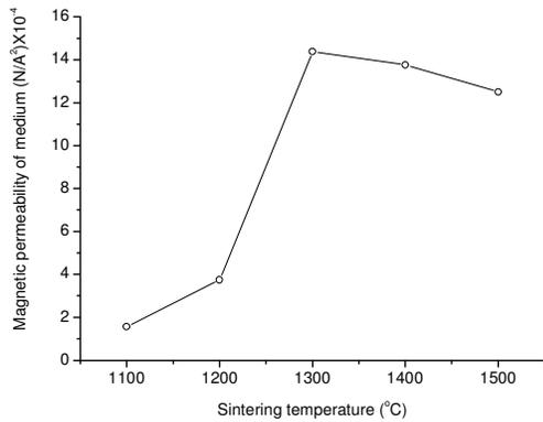
Fig. 6: The magnetic permeability medium ( $\mu$ ) of MZF ceramics sintered at various temperature.
