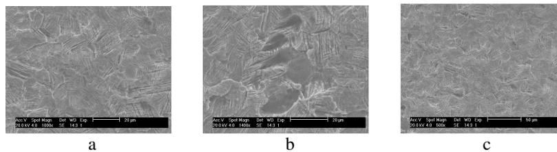
Fig. 9: Pitting in the 5.7 shot peening specimen
