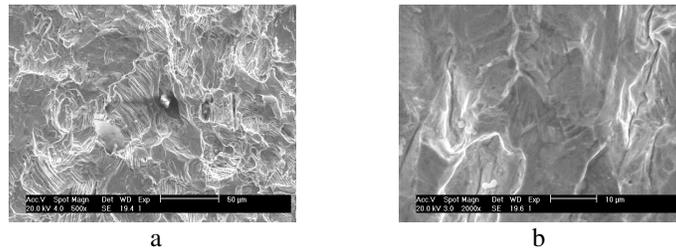
Fig. 5: Pitting and cracks for the high quality-polishing specimen
