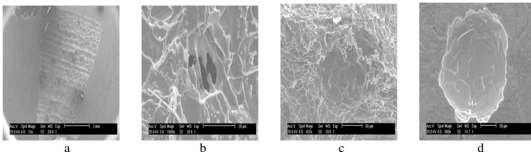
Fig. 4: Pitting and crack for 320 polishing specimen
