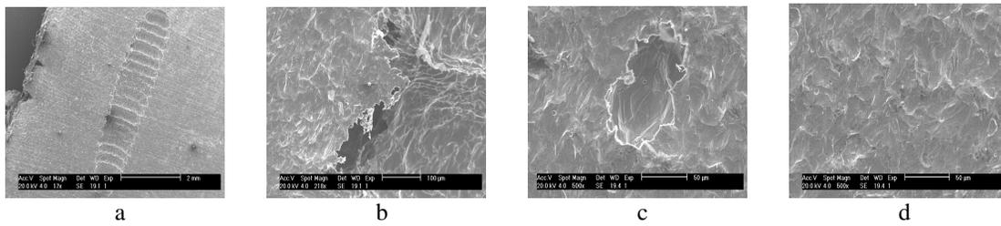
Fig. 6: Pitting and cracks for the standard polishing specimen
