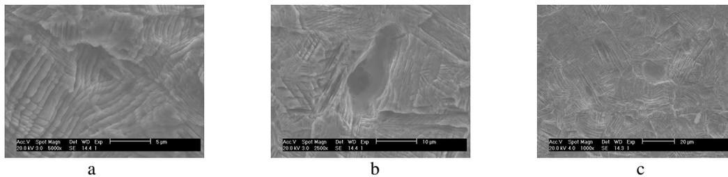
Fig. 8: Pitting in the 3.5 shot peening specimen
