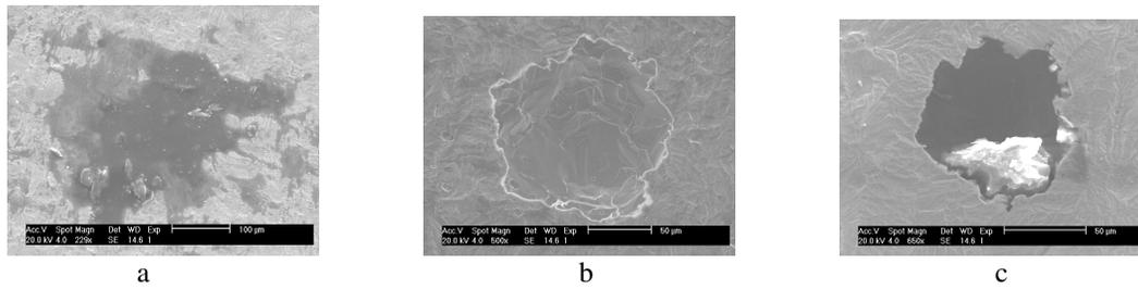
Fig. 7: Pitting in the 1.5 shot peening specimen
