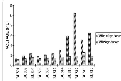
Fig. 7: Maximum over-voltages produced by a lightning stroke on bus 19
