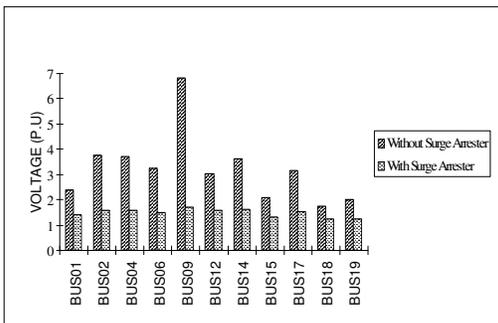
Fig. 4: Maximum over-voltages produced by a lightning stroke on bus 08
