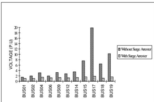
Fig. 6: Maximum over-voltages produced by a lightning stroke on bus 17
