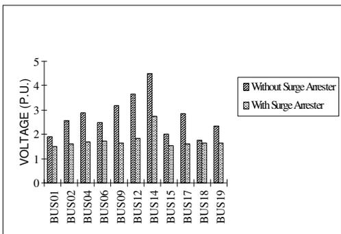
Fig. 5: Maximum over-voltages produced by a lightning stroke on bus 12
