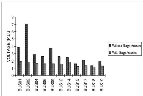
Fig. 3: Maximum over-voltages produced by a lightning stroke on bus 02
