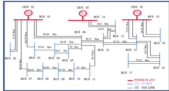
Fig. 2: Lay out of power transmission network<sup>[11]</sup>
