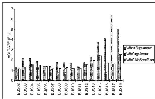
Fig. 10: Maximum over-voltages on the generator bus (Bus 18) for the three cases.
