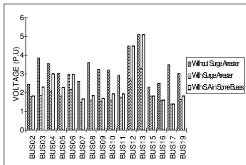
Fig. 9: Maximum over-voltages on the generator bus (Bus 14) for the three cases.
