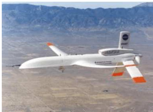
Fig. 31. ERAST is a multiyear effort to develop the aeronautical and sensor technologies for a new family of remotely piloted aircraft intended for upper atmospheric science missions. Source: (Petrescu and Petrescu, 2011)
