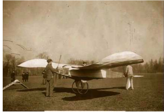
Fig. 12. The Blériot V canard monoplane, built in January 1907 Source: https://en.wikipedia.org/wiki/Louis_Bl%C3%A9riot#/media/File:Blériot_V.jpg
