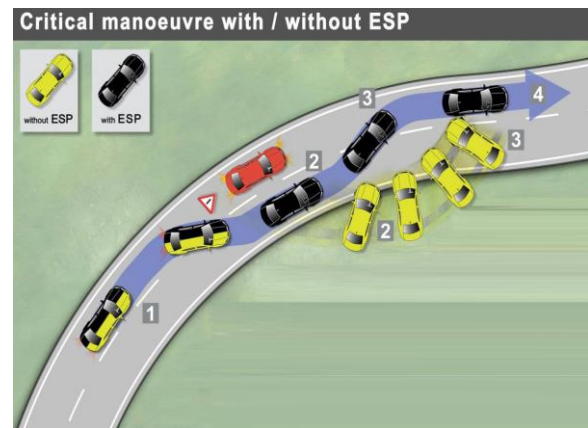
Fig. 6: Critical manoeuvre with and without EPS
