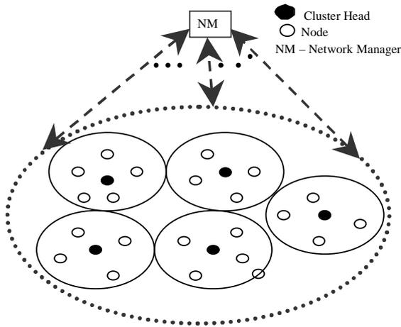
Fig. 1: Hierarchical structure of clustering model
