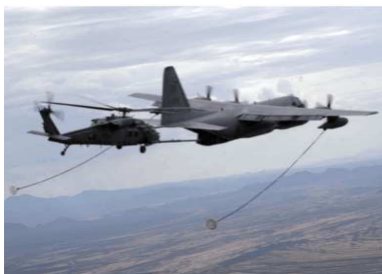
Fig. 7. USAF HC-130P refuels a HH-60G Pavehawk helicopter Source: https://en.wikipedia.org/wiki/Lockheed_C-130_Hercules#/media/File:HC-130P-N_refuels_HH-60G.jpg
