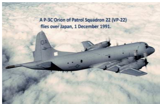
Fig. 26. Lockheed P-3 Orion is an aircraft with four motors turbo prop anti-submarine and maritime surveillance developed for the Merchant Navy of the United States Source: Petrescu and Petrescu (2013a)
