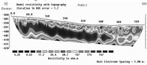
Fig. 7: The resistivity cross-section along profile 3
