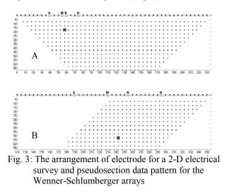
The survey was carried out using Syscal –Pro system (IRIS instruments) with 48 multi- electrodes system, with two 24 electrodes cables with 5 m electrode spacing were arranged along a profile, data level n=11 was chosen along all the profiles with 24 m investigation depth. The profile extended using a roll along technique<sup>[11]</sup>. The multi-electrodes were performed using Wenner-Schlumberger configuration. The electrodes location and elevation were measured by GPS.
