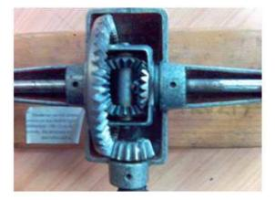
Fig. 6. A differential mechanism
