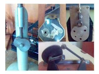
Fig. 3. Mechanisms with rotary cam and follower
