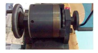
Fig. 1. Constructive photo of a harmonic drive
