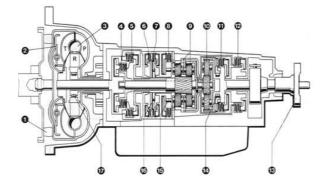
Fig. 14. An automatic transmission
