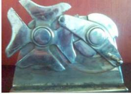
Fig. 5. A Geneva drive mechanism (Mechanism with cross of Malta), first one with one beginning and second one with two beginnings
