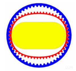
Fig. 2. Diagram of a harmonic drive
