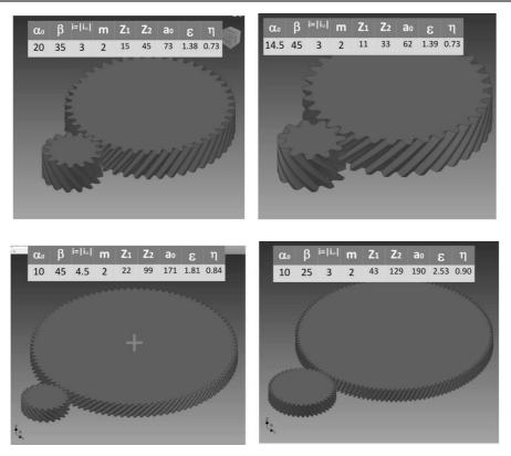
Fig. 16. Validated examples of external gearing
