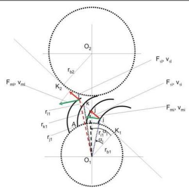
Fig. 15. Four pairs of teeth in contact concomitantly
