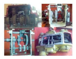
Fig. 10. Some manual gearboxes used in road vehicles
