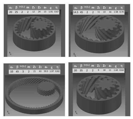
Fig. 17. Validated examples of internal gearing
