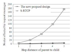
Fig. 7: Number of nodes affected by request messages in S-RTCP and ER-RTCP
