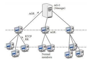
Fig. 1: Hierarchical structure of S-RTCP
