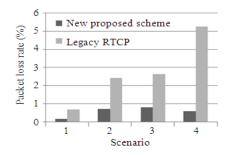
Fig. 9: Comparison of packet loss rate between legacy RTCP and ER-RTCP in different scenarios
