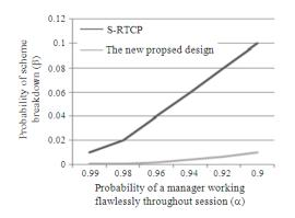
Fig. 8: Probability of scheme breakdown for S-RTCP and ER-RTCP, according to different ∝ values
