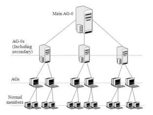
Fig. 2: The architecture of ER-RTCP
