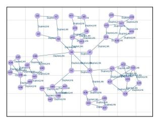
Fig. 5: Transit-stub topology used for second through fourth scenario
