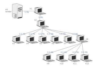
Fig. 4: The tree-shaped topology for 1st scenario
