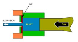
Fig. 2: Aluminum extrusion process
