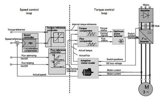
Fig. 9: Complete block diagram for Direct Torque Control (DTC)
