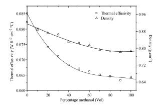
Fig. 4: Thermal effusivity and density measured at room temperature as a function of methanol in the solution
