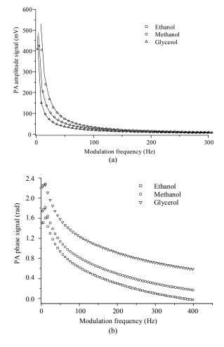
Fig. 2: The Photoacoustic signals as a function of the modulation frequency for the ethanol, methanol and glycerol. (a) Photoacoustic amplitude signal. (b) Photoacoustic phase signal
