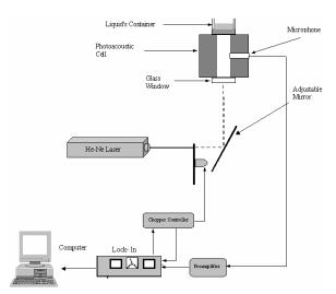
Fig. 1: Experimental setup of open photoacoutic technique
