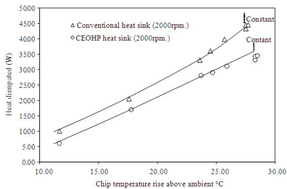
Fig. 6: Fan speed on the thermal performance of CEOHP heat sink
