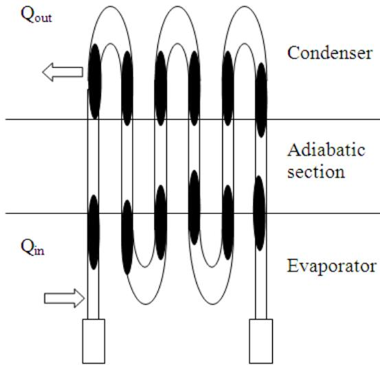
Fig. 1: Closed-end oscillating heat-pipe (CEOHP)
