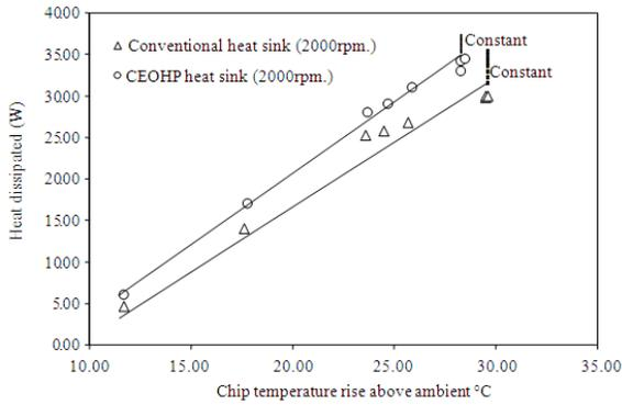
Fig. 5: Thermal performance of conventional heat sink and CEOHP heat sink
