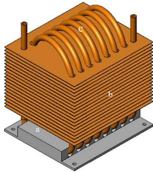
Fig. 3: Prototype: (a) aluminum base plate (b) copper fin (c) CEOHP
