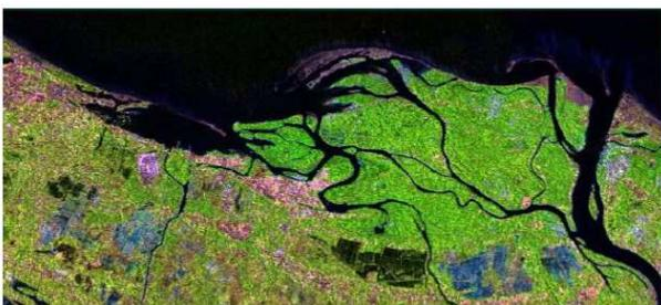
Fig. 9. SPOT5 and SAR fusion using IHS, RGB=432
