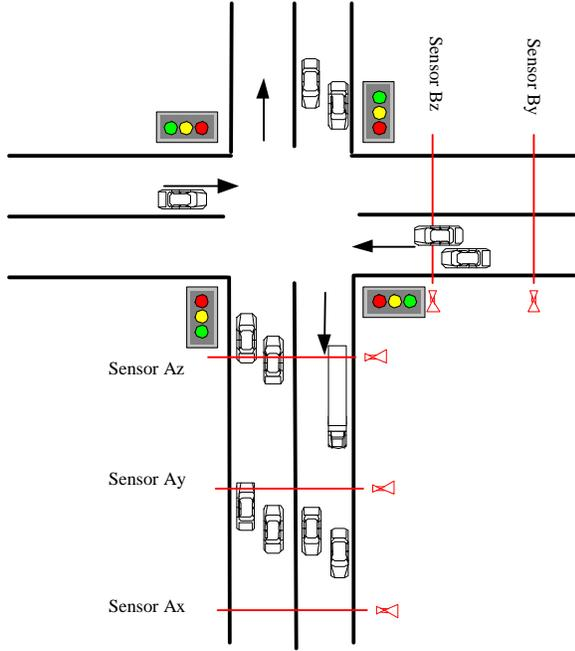
Fig. 4: RFID Reader reading range
