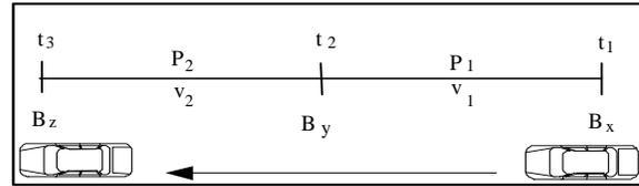
Fig. 5: Reader reading the passing through tag
