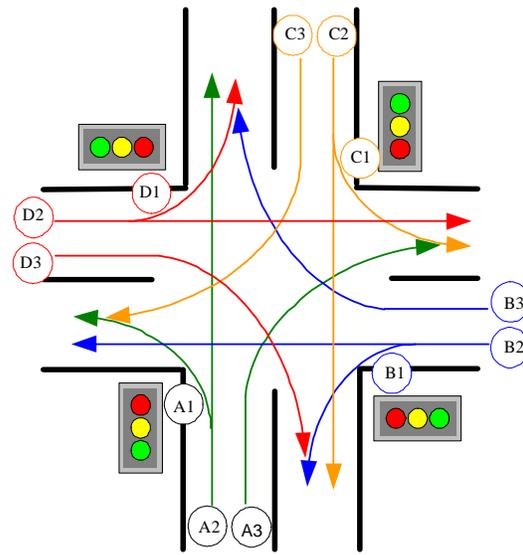
Fig. 2: Multilane traffic sequence flow
