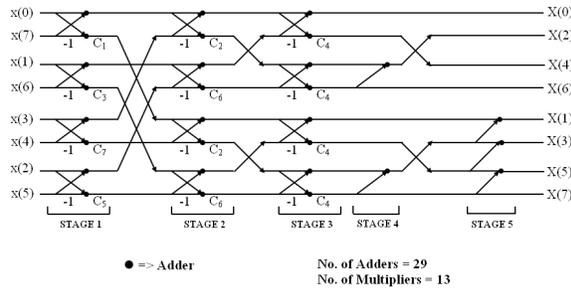
Fig. 4: Fast eight-point 1-D DCT algorithm
