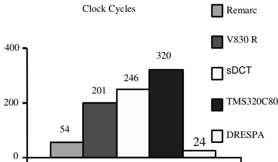
Fig. 5: Performance comparisons for 2-D DCT algorithm
