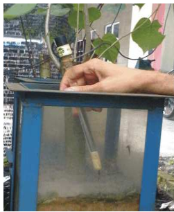
Fig. 4: A mini-tensiometer for suction testing
