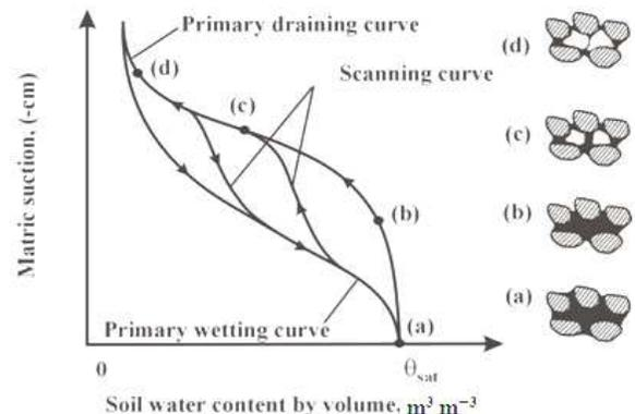
Fig. 1: The characteristics of hysteresis retention curve
