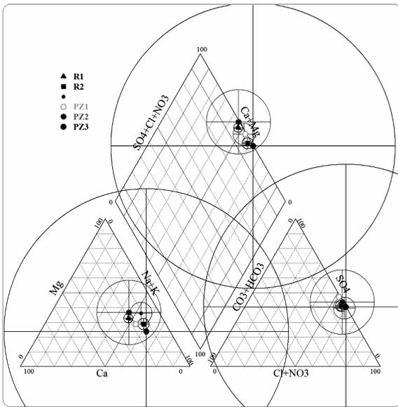
Fig. 4: The chemical facies representation in Piper diagram for discharges points and piezometers
