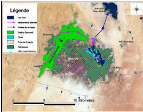
Fig. 3: The water flow in the basin of Ouargla (source: BG, 2004)
