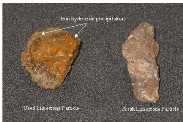
Fig. 9: Iron precipitation on limestone particles
