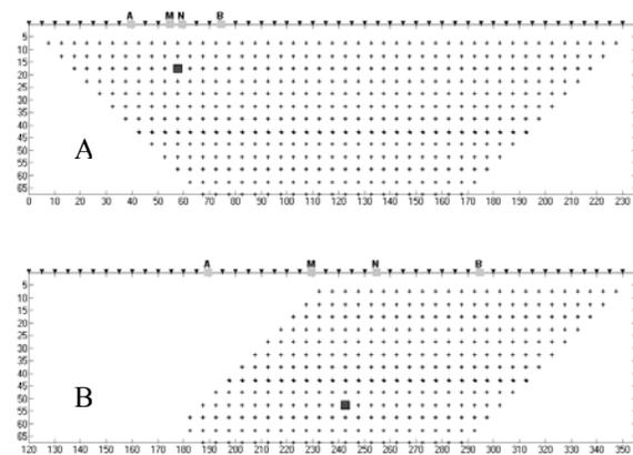
Fig. 3: The arrangement of electrode for a 2-D electrical survey and pseudo-section data pattern for the Wenner-Schlumberger arrays
