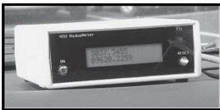
Fig. 6: Electronic display of radiusmeter (GPS method)
