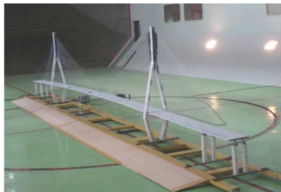
Fig. 1: The picture of the installed entire bridge model in the wind tunnel under uniform flow field
