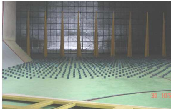
Fig. 2: The flow field simulation picture of atmospheric boundary layer type (A)
