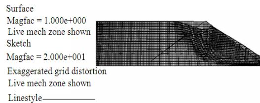
Fig. 8: Deformation after 30 sec of earthquake shaking (magnified twenty times for clarity)
