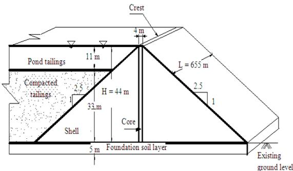
Fig. 1: Diagram of a typical tailings earthen dam
