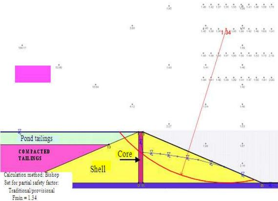
Fig. 10: Static slope stability analysis using TALREN 4
