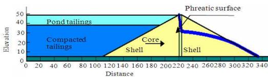
Fig. 5: Phreatic surface obtained after SEEP/W seepage analysis
