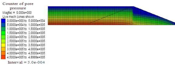
Fig. 4: Contour of pore water pressure (in  $N\ m^{-2}$ ) obtained using the FLAC<sup>3D</sup> seepage analysis
