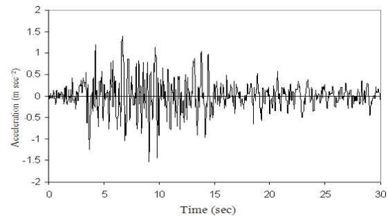
Fig. 3: Accelerogram with 1.527 m sec<sup>-2</sup> ( $\approx 0.15$  g) peak horizontal acceleration applied at the base of the dam
