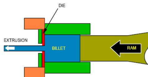
Fig. 2: Aluminum extrusion process
