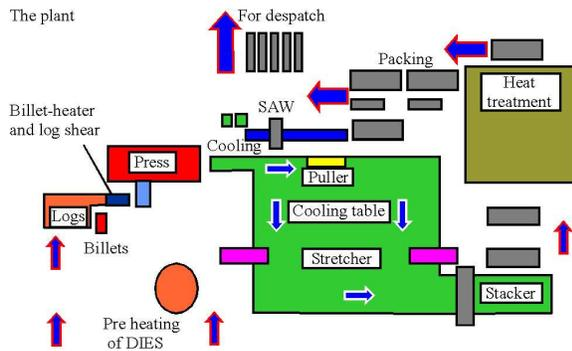
Fig. 3: Layout of a typical extrusion plant
