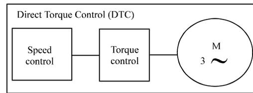
Fig. 8: Control loop of an AC Drive using DTC
