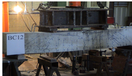
Fig. 9: Crack propagation and failure of the beam under load
