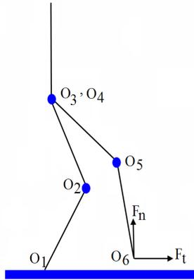
Fig. 2: Considering closed kinematic chain of biped to be opened in double support phase.
