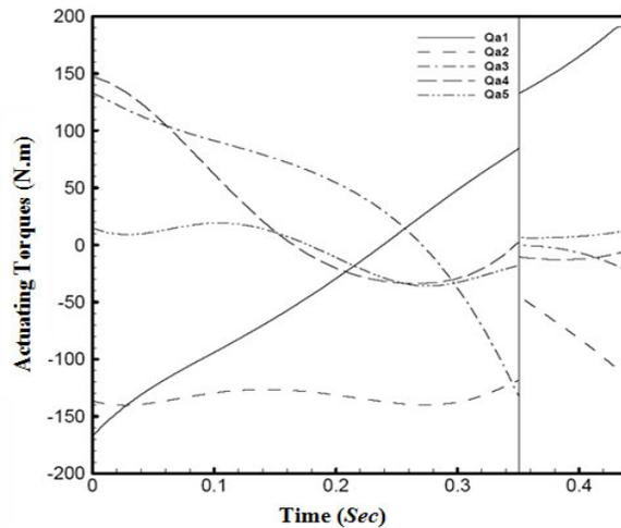
Fig. 5: Time variation of actuating torques.
