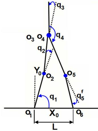
Fig. 1: Biped kinematic model.
