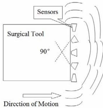
Fig. 3: Proposed sensor assembly on the surgical tool.
