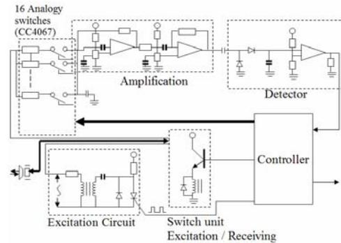
Fig. 5: Various circuits of the signal processing system.
