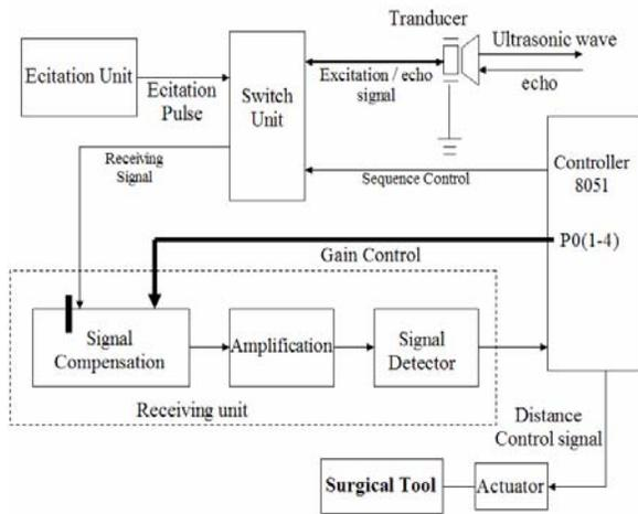
Fig. 4: Block diagram of the signal processing system.
