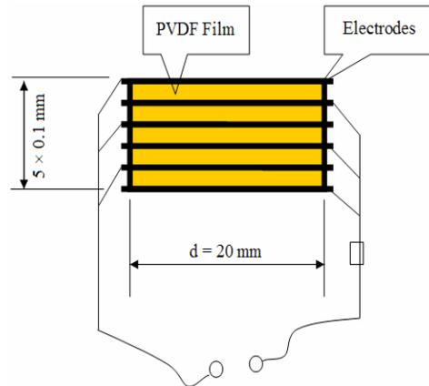
Fig. 2: Transducer configuration.
