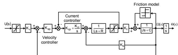
Fig. 10: Detailed model of rotary positioning system
